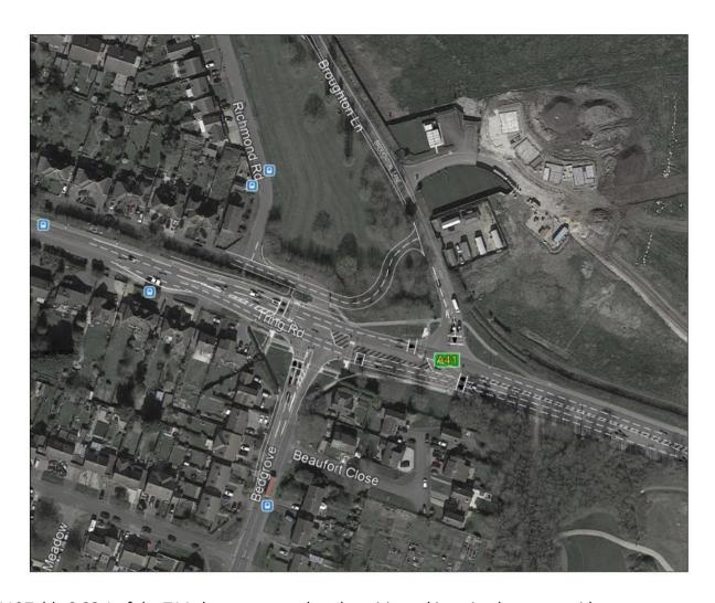
5.119Table 3.22.1 of the TAA demonstrates that the mitigated junction layout provides a significant level of betterment over the 2036 Do Minimum situation, with the junction operating within theoretical capacity in both scenarios and significant reductions in mean maximum queues.
