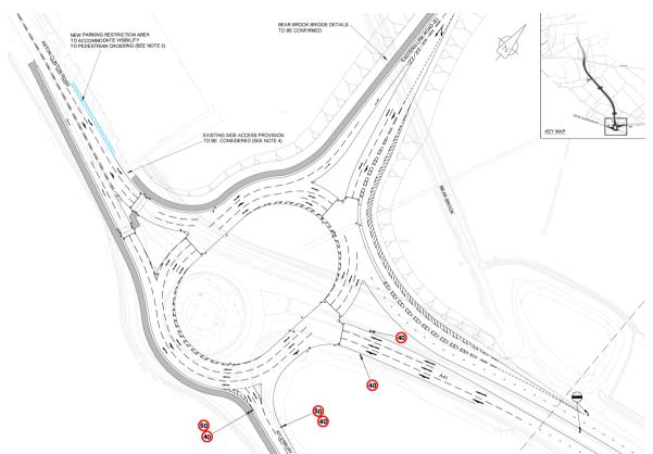
5.108 The results of the 2022 Do Something scenario based on the layout above are set out below and show that the junction would operate within capacity with the standalone Woodlands first phase of development. The key assessment criteria are the degree of saturation (DoS/RFC) and queue. A junction is indicated as being within capacity where the DoS/RFC is at or below 85% for priority junctions (including roundabouts) and 90% for signal controlled junctions.
